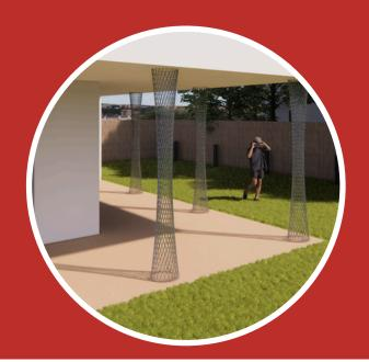
Innovative lattice pole with a rhomboidal structure, formed by interconnected lateral faces projecting a polygonal shape. The pole, developed vertically with interconnected rhomboidal lattice elements, is manufactured using WAAM (Wire and Arc Additive Manufacturing) technology in a "dot-by-dot" or "point-by-point" method.
